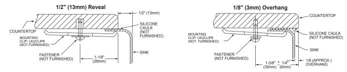
NOTE: THIS UNDERMOUNT SINK IS DESIGNED TO MOUNT TO SOLID SURFACE (NON-LAMINATE) COUNTERTOP ONLY.
