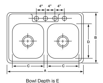
Hole Drilling Configurations
